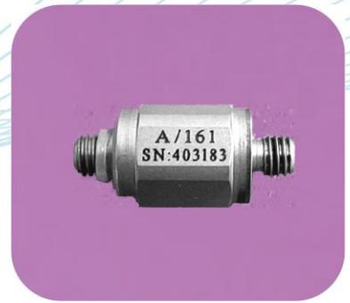
Developed for demanding applications requiring the measurement of high amplitude, short duration transient events such as pyrotechnic shock or high energy impacts, the A/16X range of stainless steel IEPE accelerometers have a range from 10,000g up to 50,000g
